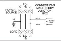
In 230 VAC installations, one side of the line going to the load is always HOT. This condition exists if the switch is on or off. Install double pole disconnect on all 230 VAC circuits.
