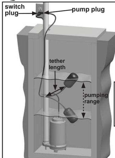
*Due to weight of cable, pumping range above horizontal is NOT equal to pumping range below horizontal. Use values published on front page as a guide. Pumping ranges are based on testing in non-turbulent conditions. Range may vary due to water temperature and cord shape. Note: As the tether length increases, so does the variance of the pumping range.*
